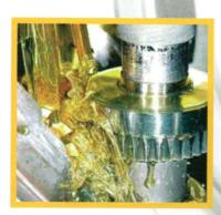
**Powercut A12 Premium** is a non-staining type neat cutting oil blended from high VI base oils fortified with chlorinated EP additive and is free flowing, giving better heat dissipation characteristics. This oil is suitable for machining of aluminium components.
