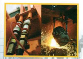
**Fire Resistance Hydraulic Fluid : (HFD-U type) POWER SAFEFLUID SE 46 & 68** are based on high quality synthetic organic esters and selected additives. POWER SAFEFLUID SE replace anti wear mineral oil fluids when fire hazards exist and in environmental sensitive applications.
